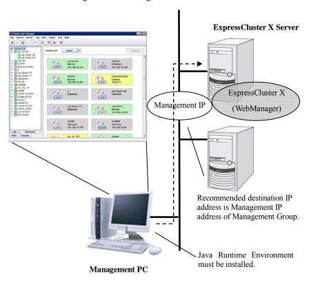
There are two types of the Integrated WebManager: the Java applet version that operates on a Web browser, and the Java application version that can be operated by installing on a management PC and executed on Java Runtime Environment (JRE).
